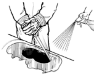
Hand Sawing Asbestos Cement Pipe
